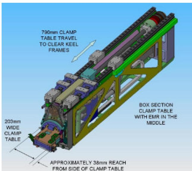
Figure 16: Inner Machine Head
