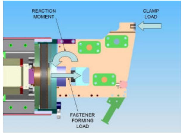
Figure 11: Offset Fastening Loads
