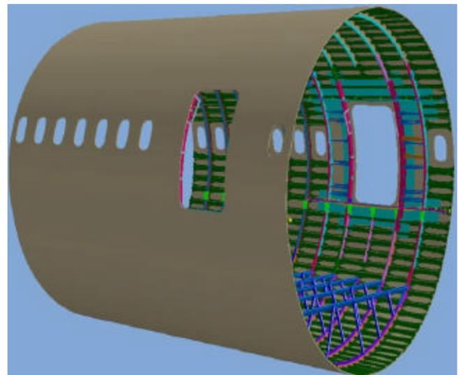
Figure 2: Boeing 787 One Piece Barrel (OPB) Design
