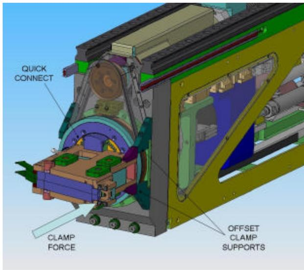
Figure 13: Clamping Loads
