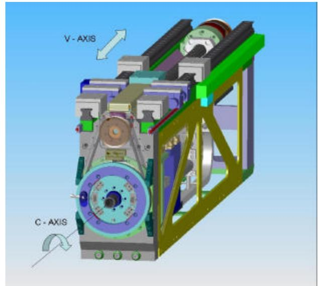
Figure 8: Inner Machine True Offset Head
