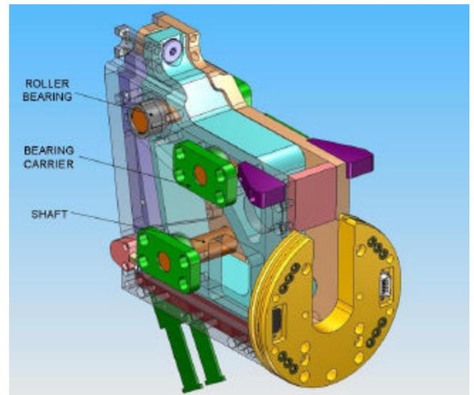
Figure 14: Offset Fastening Support Bearings
