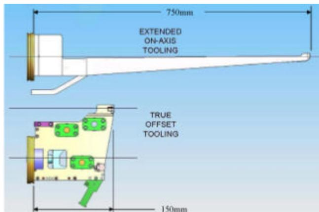
Figure 4: Traditional tooling vs. True Offset Tooling
