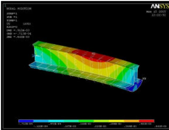
Figure 19: Inner Floor FEA results (Y-axis)
