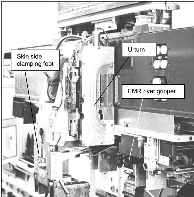
Figure 3. Rivet U-turn on pre-SA2 LVER machine.
