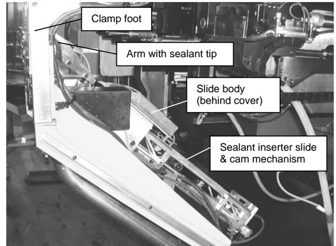
Figure 6. SA2 sealant inserter.
