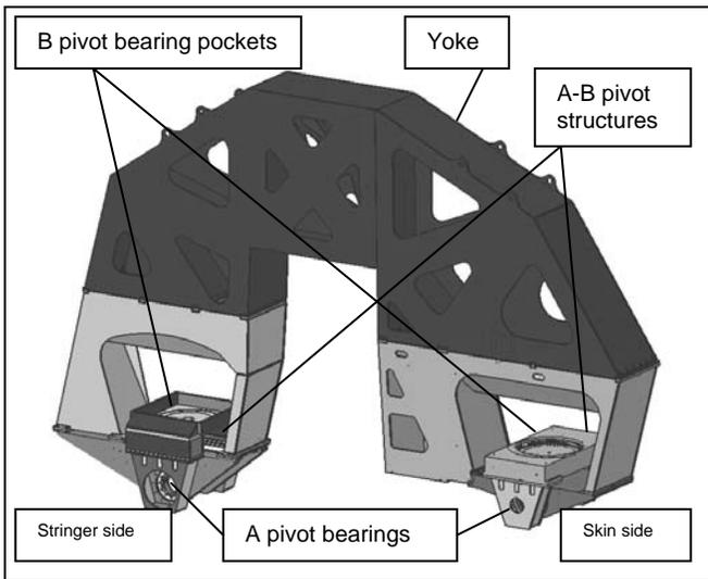
Figure 11. LVER yoke, generation 4 (pre-SA2).
