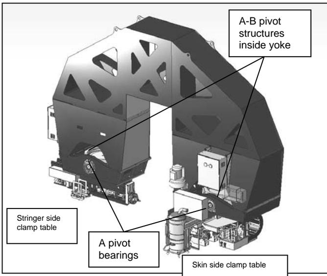
Figure 12. LVER yoke, generation 5 (SA2).
