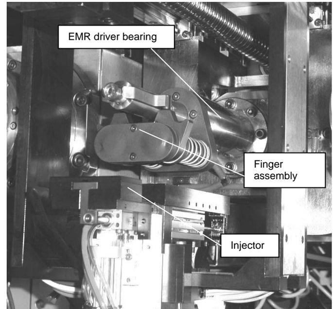
Figure 4. SA2 rivet fingers and injector on EMR.
