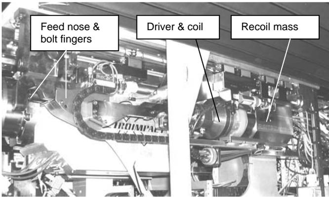
Figure 7. Electromagnetic bolt insertion tool (EMB).
