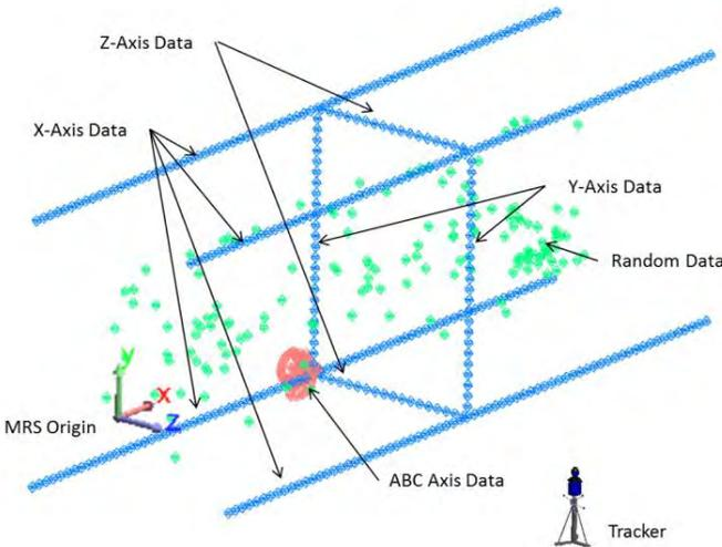
Figure 10 – X, Y, Z, A, B, C and Random Compensation Data
