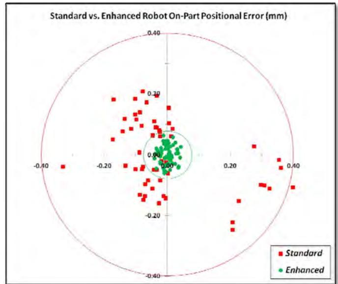
**Figure 3. Accuracy comparison: Standard vs. Enhanced**
