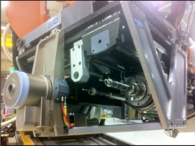
**Figure 4. Multi-function end effector. Left to right: nose piece, camera, hole probe, spindle**
