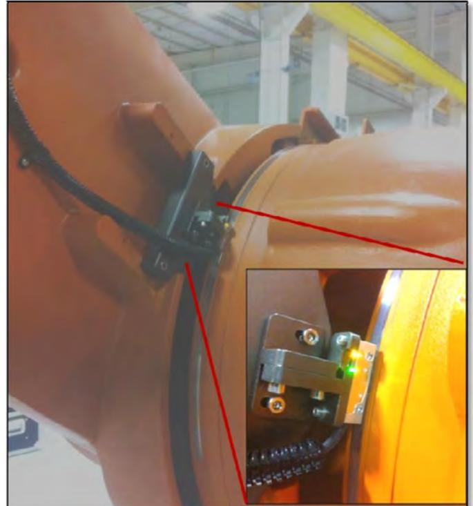
**Figure 2. Secondary encoder mounted to output of robot axis**
