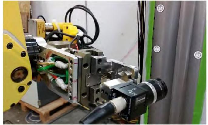
Figure 19. Robotic Vision testing using a camera held in the M10 EOAT sighting three targets.
