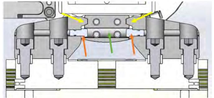
Figure 11. M20 EOAT gripper finger wedge and backup pin cross-section.
