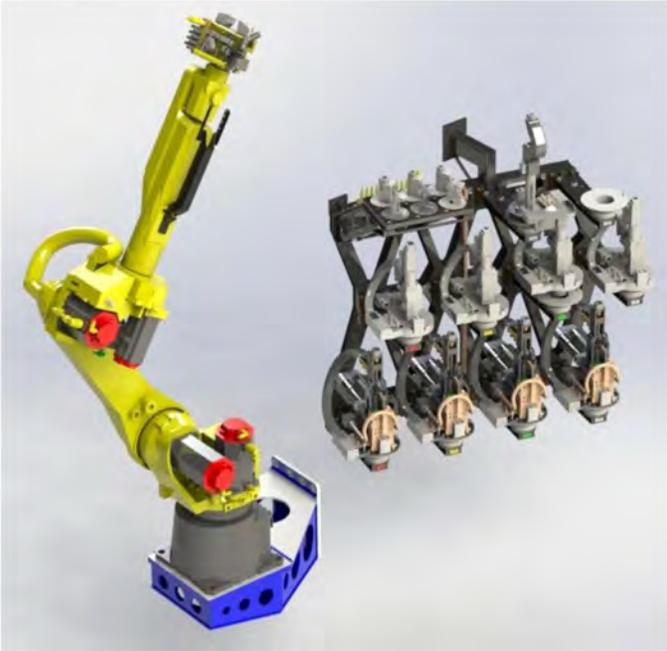
Figure 8. M20 robot with nosepiece rack.
