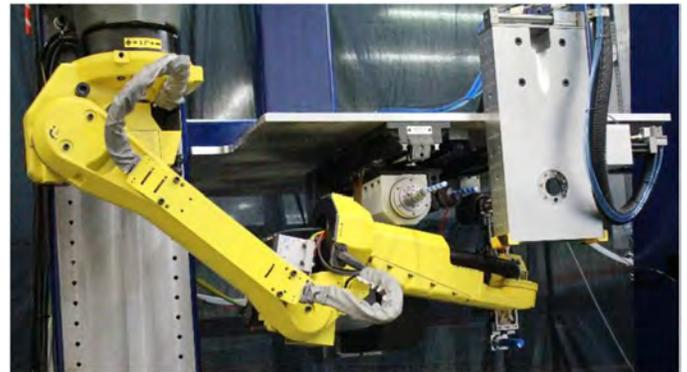
Figure 17. M10 robot in position for a close clearance pick on ATC testbench.
