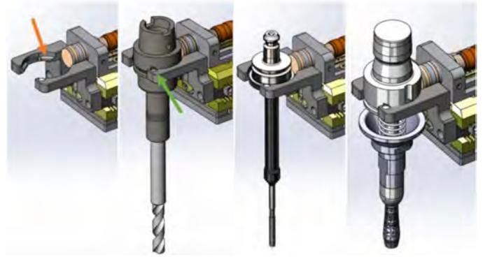
Figure 2. M10 EOAT in various states. Left to right: empty, gripping drill bit, gripping hole probe, gripping bolting anvil. Note all tools mate with the same gripper locating taper (orange arrow) and clocking dowel (green arrow).
