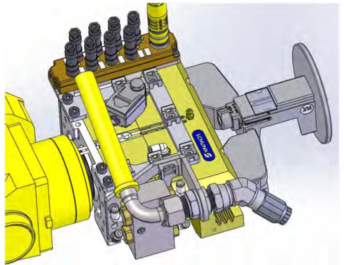
Figure 3. 3/16" vacuum nosepiece in M20 EOAT
