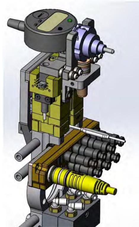
Figure 20. Plunger gage alignment tool in M10 EOAT.
