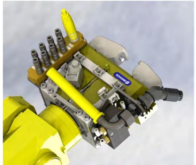
Figure 10. M20 robot EOAT
