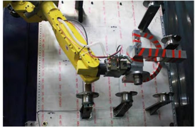
Figure 14. M20 robot reaching to the collar swage / nutrunner / vacuum nosepiece tool rack during high payload testing.
