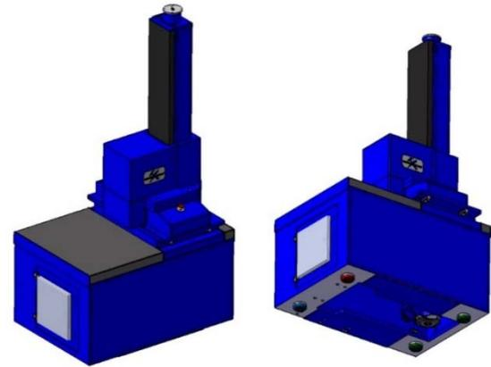
Figure 12: Single positioner module of the APS. Foundation cup/cone interface (right).
