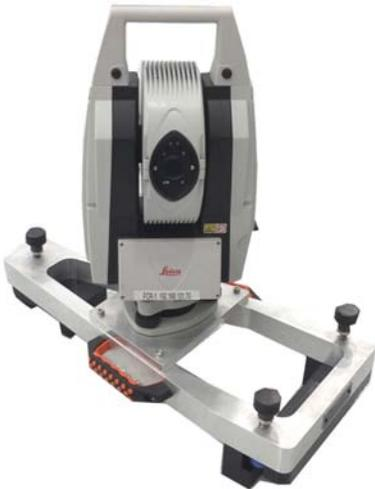
Figure 19 A custom stand is used to mount the tracker on the a/c seat track rails.
