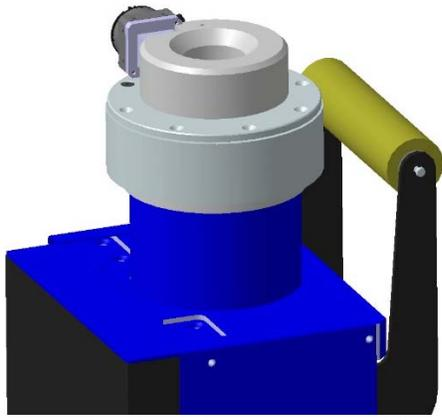
Figure 13: Custom handling ball receiver. Lateral float with lockout. Ball sensing and retaining. Spring actuated and pneumatically released in a tight package.
