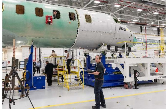
Figure 5 Forward fuselage join is achieved via feedback from tracker mounted inside the fuselage. Photo credit: Robert Backus.
