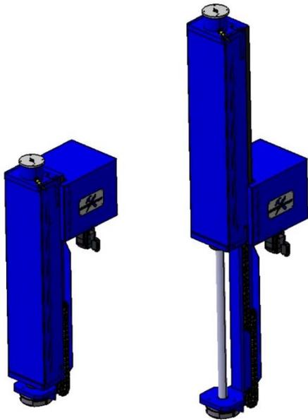
Figure 11: Example compressed and extended heights of APS vertical axis
