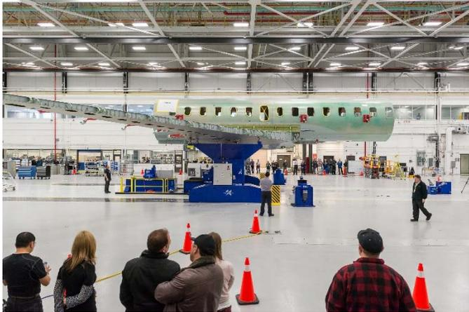
Figure 6 ATLAS moves the wing-fuselage section to the next workcenter. Center of mass is surprisingly far back in the assembly. Photo credit: Robert Backus.
