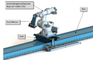
Figure 3. Primary Axis Components
