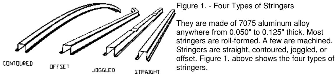
Joggled and offset stringers generally require extensive tooling to accommodate their irregular geometries. However, the majority (approximately 75 - 80%) of the stringers to be drilled for the 747 fuselage are straight or contoured. Therefore, simple, easy-to-use tooling effective for straight and contoured stringers was preferred to a complex system compromised for holding irregular stringers.
