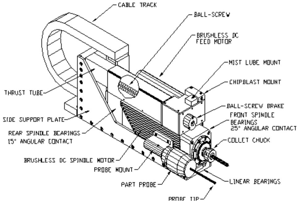
Figure 3. - Model 04 Servo-Servo Drill
