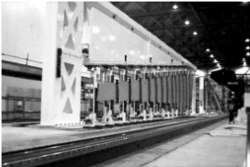
hole drilling. The U side head presses the panel up against the fixture. The inboard pattern is employed when the wing panel is attached to the center wing box.
