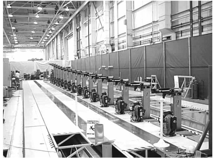
Figure 5: Flexible Fixture Unloaded
