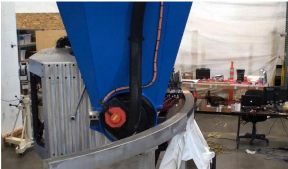
**Figure 5 – Electroimpact seven axis AFP machine with swing-through head**
