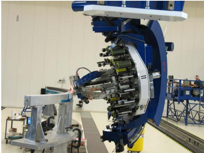
**Figure 2 Cprime rotation during laydown**
