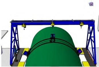
Once the EFT's are deployed the GHS is rolled away and stored. Lastly, four more sections of rail are spliced at each end of the 10 track sections loaded from the GHS.
