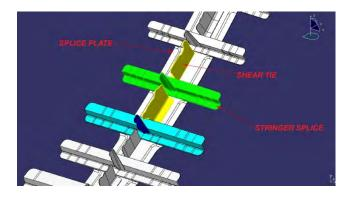
Figure 2. 777 – Buttsplice Components (Detail)
