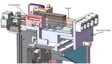
Figure 4 - Muzzle, Through beam and Feed tube shifter
