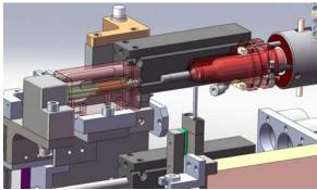
Figure 11 - Bolt held by bolt inserter fingers
