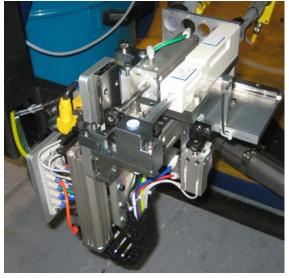
Figure 1- Pinch bolt injector E4380 #9 with 1/4" feed tooling
