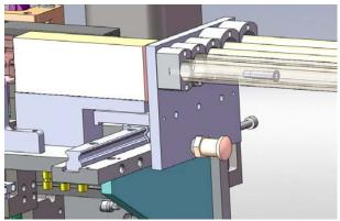
Figure 5 - Bolt in feed tube
