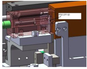
Figure 8 - Stop Pin extended
