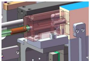
Figure 7 - Bolt breaking fiber optic beam
