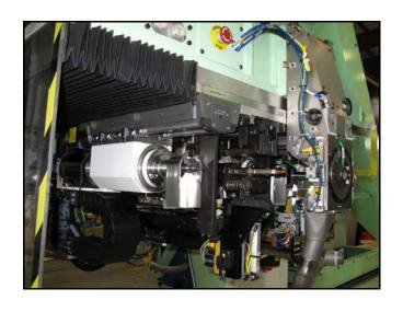
Figure 12: E6000 clamping foot and process tools.
