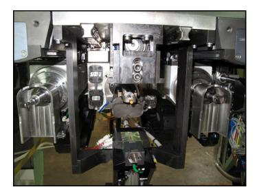
Figure 11. Drill spindle, EMR, and shave spindle. All are servo-actuated.
