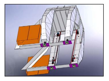
Figure 6. Rigid gantry structure.
