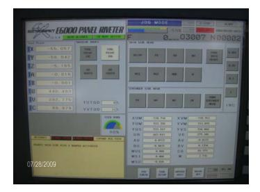
Figure 17: CNC display in Jog mode.
