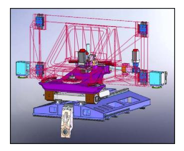
Figure 7. Skin side Y-A-B-U assembly, process tools not shown.
