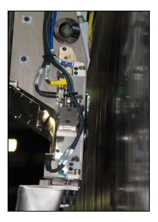
Figure 15: E6000 machine with laser normality sensors follows a test panel's curvature.
