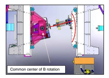
Figure 4. Coordinated head motion at B = 12°.
