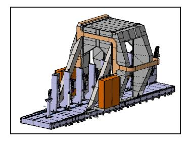
Figure 9. Machine and fixture on monolithic bed structure.
