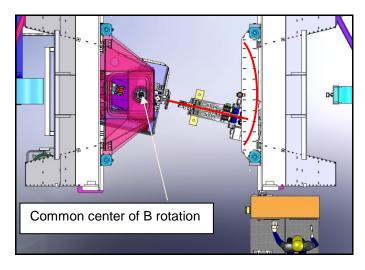
Figure 5. Coordinated head motion at B = -12°.
