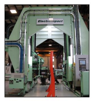
Figure 1. E6000 riveting machine.
