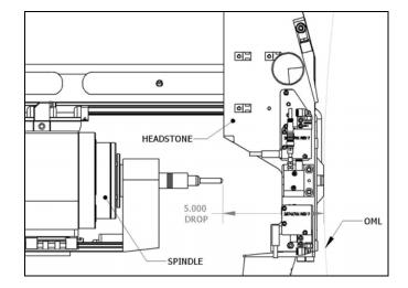
Figure 13. Depiction of 125 mm / 5" drop on E6000. Drill spindle, shown in retracted position, traverses this distance to reach the panel.
