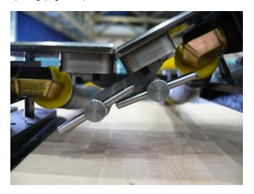
Figure 6. Quick Change Track Splice
