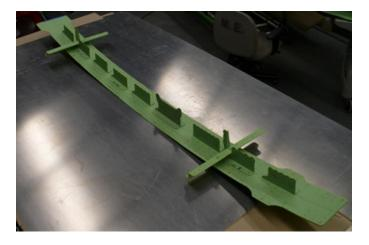
Figure 2. Subassembly of splice plate, shear ties & stringer splices
