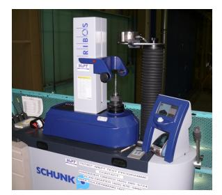
Figure 4. Tool Presetter
