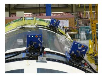
Figure 1. Flex Track Drilling Machines on 777 Fuselage
