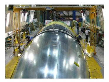
Figure 5. Gantry Handling System
