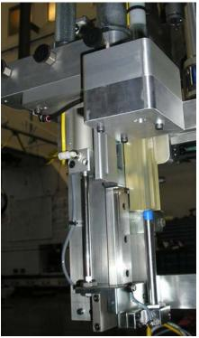
Figure 2 push bolt injector
