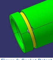
Figure 6: Socket Detent
