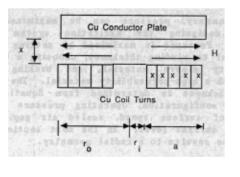
= permeability of spacex = gap thicknessN =number of turnsn=coil turn density=N/a
