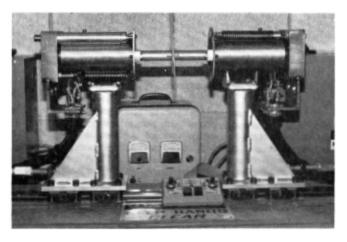
Plate 1: Prototype Model of the Robotic Actuator
