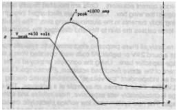
Figure 4 Voltage and Current Pulses for the LVEIDI Module Conclusion
