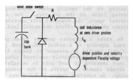
Figure 2 Capacitor Discharge Circuit
