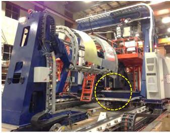
Figure 7. Machine parked, showing the lower beam tucked under the notch in the fixed positioner tower
