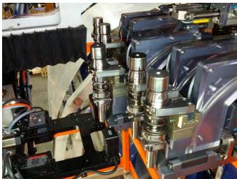
Figure 11. Injector-mounted automatic anvil tool changer
