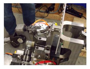
Figure 9: Rivet is advanced in the fingers
