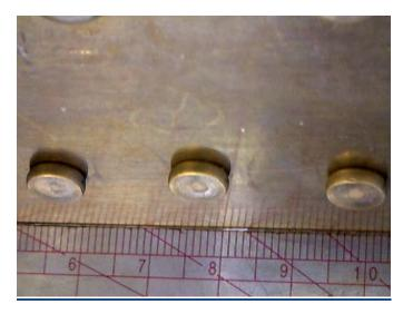
Figure 12: Formed tails of 3/16 universal head rivets are consistent
