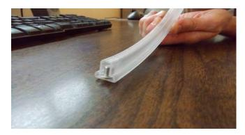
Figure 6 Rivet is blown down a shaped tube to prevent tumbling
