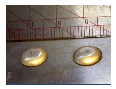
Figure 11: Heads of 3/16 universal head rivets are consistent
