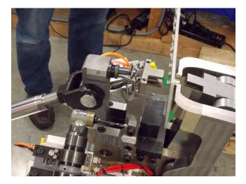
Figure 10: Unclamp after the rivet is formed
