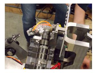
Figure 7: Clampup and drill to breakthrough position
