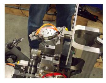
Figure 8: Rivet is fed into the rivet fingers
