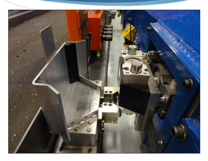
• Automated indexes provide solid union between machine and jig
