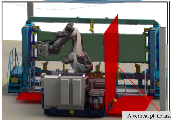
A vertical plane laser scanner keeps the robot from extending beyond the side of the platform and reduces the size of the restricted space
