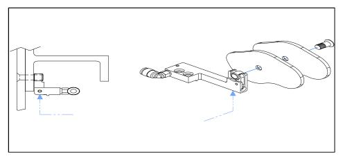
Figure 17: gripper finger opened and collar released
