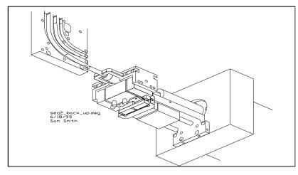
Figure 5: sequence of operation for the rivet gripper #2 showing 1" gap
