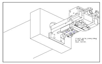
Figure 3: rivet gripper assembled
