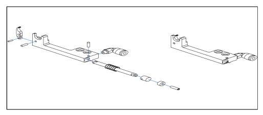
Figure 12: collar gripper (exploded)
