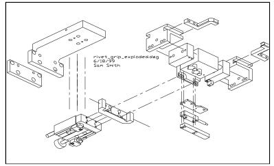
Figure 2: Exploded view of rivet gripper assembly
