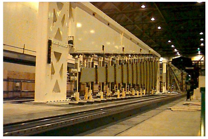
Figure 1: automated riveting machine on 8' x 50' wing panel
