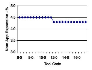
Figure 6 - Nominal Applied Expansion Levels for CMX Process.
