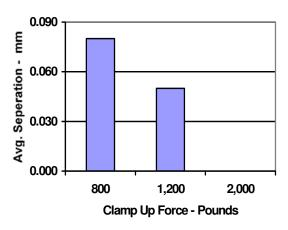
Figure 4 - Stackup separation vs. clampup forces
