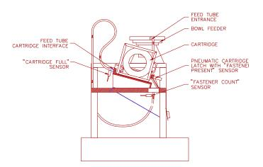
Figure 6. Filling Station Layout
