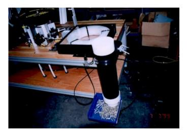
Figure 7. Manual cartridge purge station
