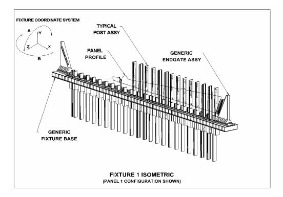
Figure 2: Flexible "Popping Post" Fixture
