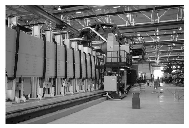
Figure 7: A340-600 Upper Panel Line: Tack Pass Note: Skin strap push panel into correct contour.
