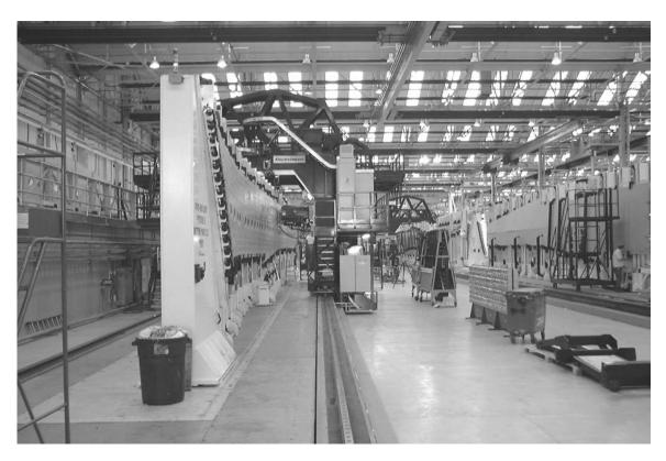
Figure 6: A340-600 Lower Panel Line: Fill Pass with E4100 Assembly machine
