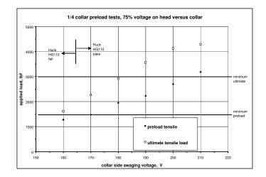
Figure 6. 1/4 Collar Pre-load Tests
