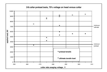
Figure 8. 3/8 Collar Pre-load Tests
