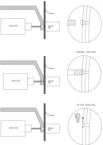
FIGURE 5 – RIVET SHAVING PROCESS
