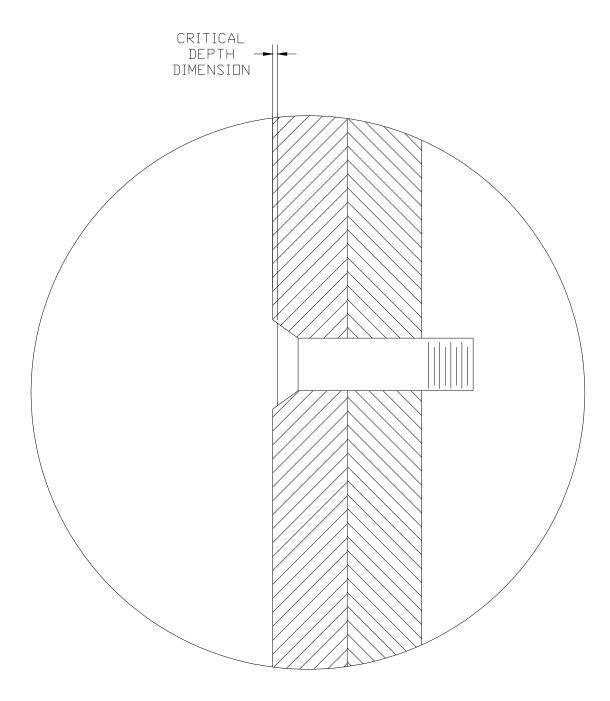
FIGURE 4 – TYPICAL INSTALLED BOLT
