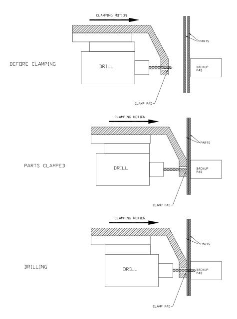
FIGURE 1 – DRILLING PROCESS
