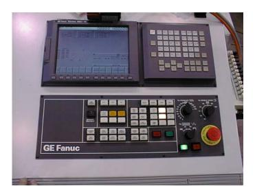
Figure 3: DDEE Fanuc 18i Controller
