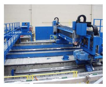
Figure 1: Gantry Drill Machine (Floor covers not installed)
