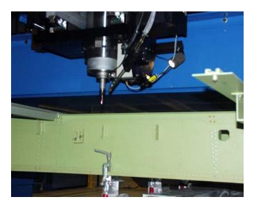
Figure 7: Coolant Application on Tool
