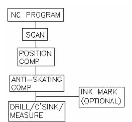
The system process begins with the off-line generation of NC programs. The Cell Control executes NC programs that are generated with custom software built around IGRIP, a robotics simulation and off line programming software package available from Delmia Corp. The TEF is then loaded into the holding fixture.
