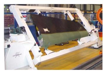
Figure 8. Holding Fixture
