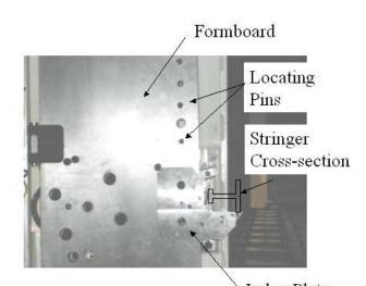
Figure 3: Prototype A380 pegboard ("formboard") and one index-plate
