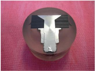
Figure 5 – Sectioned mold
