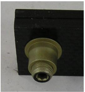
Figure 2. Tail view of 3/8 pin with CT collar
