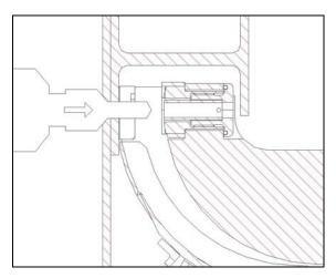
Figure 6 - Step 2: Ram pulls back to allow drill breakthough
