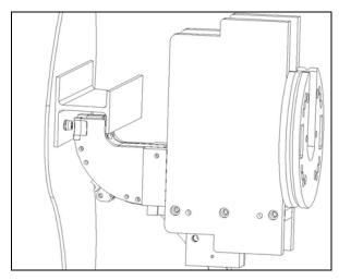
Figure 12 - Step 8: Strip die off of collar and unclamp
