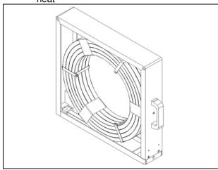
Figure 4 - Collar cartridge assembly
