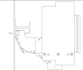
Figure 5 - Step 1: Machine clamps up at a location
