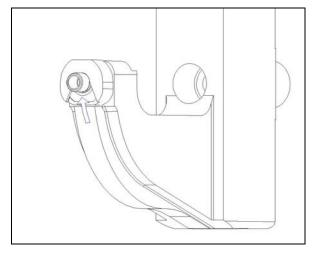
**Figure 8 - Step 4:** Collar is fed transverse through slot to sleeve. Sleeve has v-notch alignment feature to locate the collar
