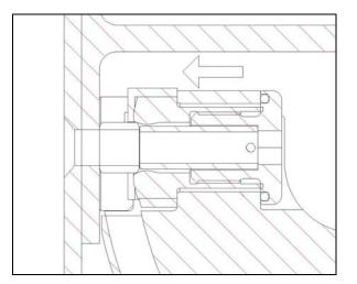
**Figure 9 - Step 5:** Ram moves toward work to capture collar against work piece in the bell-mouth of the die. Collar position and orientation verified via linear potentiometer
