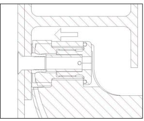
Figure 11 - Step 7: Swage collar with EMR
