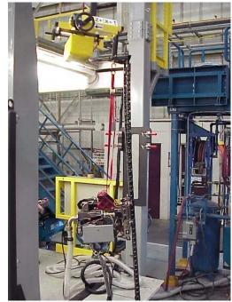
Figure 16: Vertical Handling with Adjustable Counterbalance
