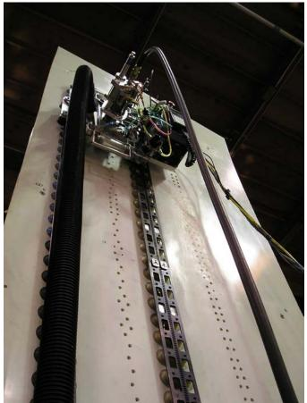
Figure1: Prototype Flex Track
