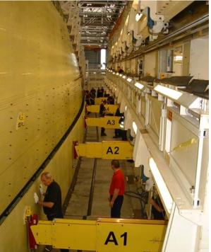
Figure 1, Panel supported by Panel Loaders in wing form prior to engagement with sub-structure.
