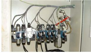
Figure 6, Hydraulic manifold typical each arm.
