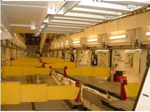
Figure 2, Eleven Panel Loader arms deployed on 2<sup>nd</sup> level empty starboard jig.
