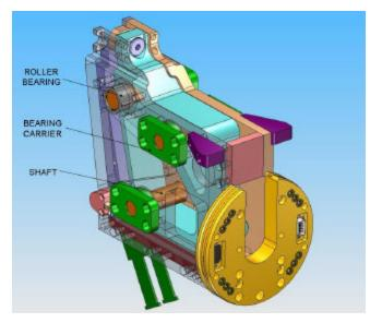
Figure 14: Offset Fastening Support Bearings
