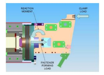
Figure 11: Offset Fastening Loads
