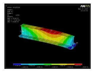
Figure 19: Inner Floor FEA results (Y-axis)
