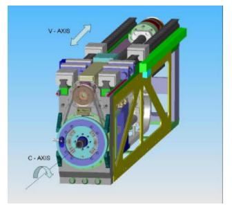
Figure 8: Inner Machine True Offset Head
