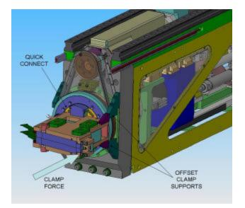
Figure 13: Clamping Loads
