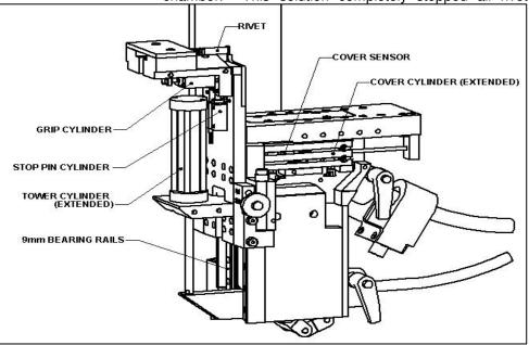
Figure 5: Diagram of the rivet injector in the raised position
