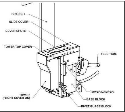
Figure 3: Diagram of the major components comprising the rivet injector
