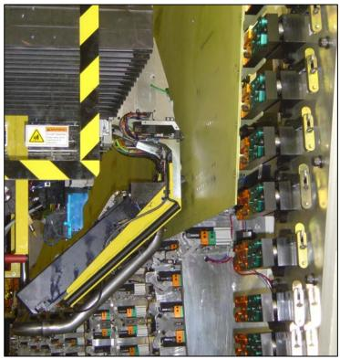
Figure 2: The skin side process tools and clamping foot. The rivet injector is the blue rectangle left of center.
