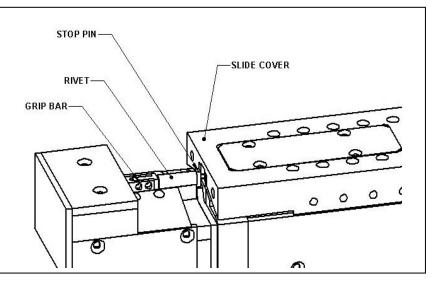
Figure 4: Diagram of the rivet chamber showing the rivet griped between the stop pin and grip bar
