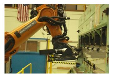
Figure 2. 737 Aileron Robot working with an existing jig.
