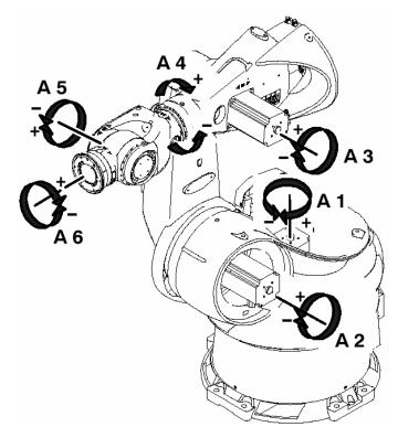
Figure 3. KUKA Robotics KR 360/2 Robot.
