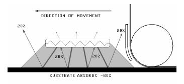
Figure 4. Undesirable Reflected IR and Waste Heat
