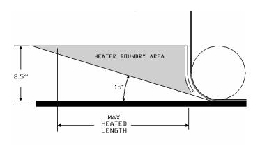
Figure 1. Heater Geometry Constraints
