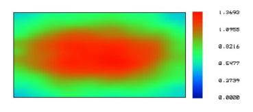
Figure 3. Irradiance on Target Plate
