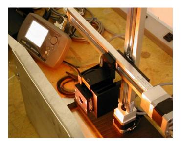
Figure 7 Power Meter on X/Y Stage Measuring Irradiance
