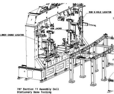
The Lower Chord tooling indexes and clamps the Lower SOB chord in position, while allowing each individual index to be either dropped for access, or indexed at an offset for inspection measurement. The SOB Ribs are indexed using an air powered jacking system and aligned with pins through the coordination holes. The stationary base also provides access at an optimum work height for technicians, as well as easy access to the inside of the Section 11.
