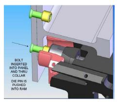
Figure 12: Bolt and collar position check
