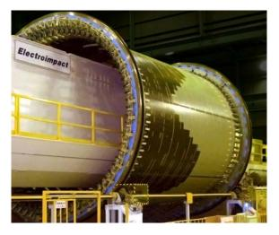
Figure 2: Boeing 787 One-Piece-Barrel (OPB)
