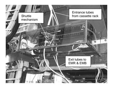
Figure 8. SA2 fastener buffer.
