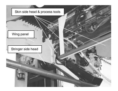
Figure 2. LVER machine fastening heads.
