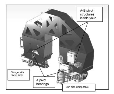
Figure 12. LVER yoke, generation 5 (SA2).
