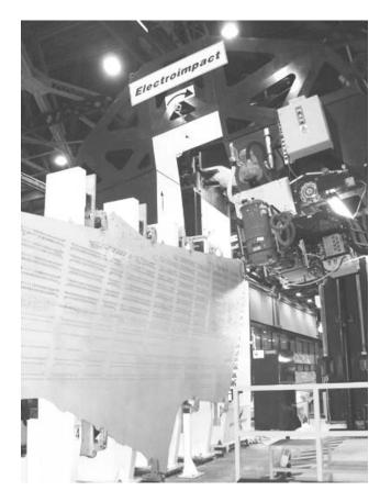
Figure 1. SA2 wing panel fastening machine.
