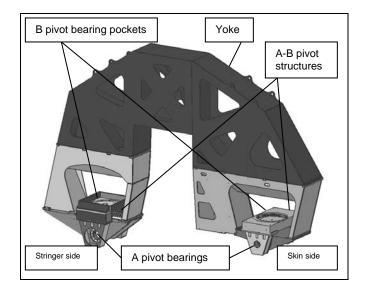
Figure 11. LVER yoke, generation 4 (pre-SA2).
