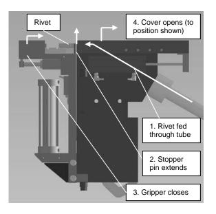
Figure 5a. Rivet feed sequence to injector.
