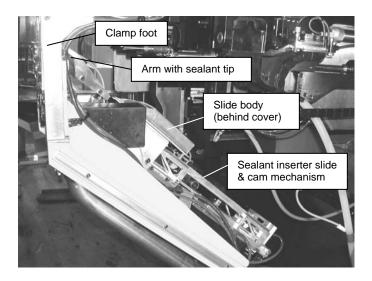
Figure 6. SA2 sealant inserter.
