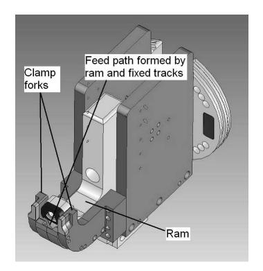
Figure 9. Anvil for offset collar installation.
