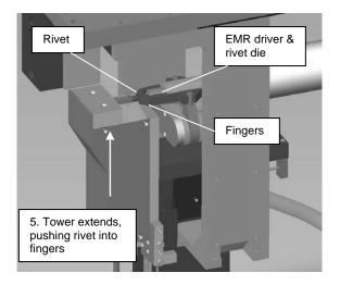
Figure 5b. Rivet is fed into EMR fingers.
