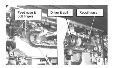
Figure 7. Electromagnetic bolt insertion tool (EMB).
