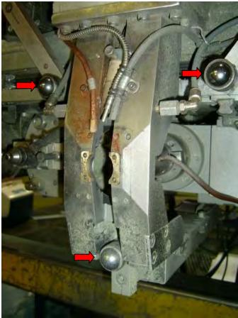
Figure 3 - Head stone with normality sensors
