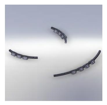
Figure 6 - B axis bearing arrangement
