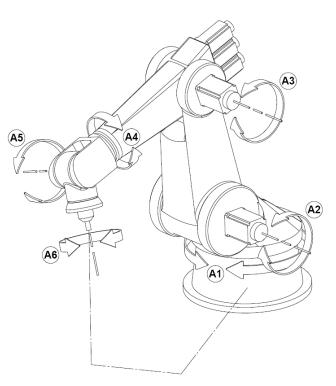
Figure 1. Typical serial link 6-axis robot
