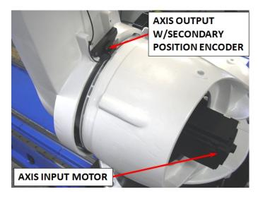
Figure 4. Applied secondary feedback at joint output
