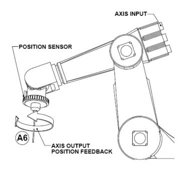
Figure 3. Secondary feedback at joint output
