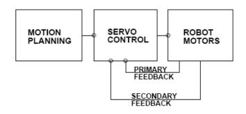
Figure 5. Direct use of secondary feedback
