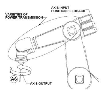
Figure 2. Standard location for position feedback
