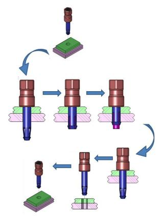
Figure 1. Using a single-sided slave fastener
