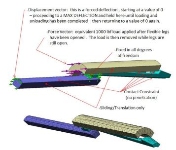
Figure 25. Model and meshing for Case 2 loading
