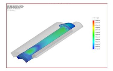
Figure 27. Maximum stresses during clamping – top view.
