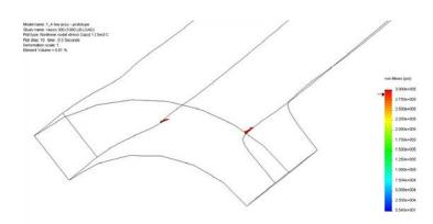
Figure 28. Volume of material that has exceeded yield levels.
