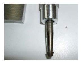
Figure 38. The tool is reverse torqued until it returns to its neutral state. Notice that the fingers are touching at the tips. This suggests than no noticeable residual
