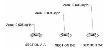
Figure 21. A single finger for a typical  $\emptyset$  1/4 inch SSSF is shown in the post heat treat condition; multiple section planes are shown.
