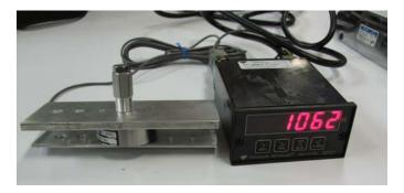
Figure 37. The tool is torqued until the load cell reads approximately 1000 lbs (a little over to account for any error) which corresponds to the Load Case 2 in the FEA section.
