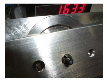
Figure 39. The tool is torqued until the load cell reads approximately 1600 lbs (a little over to account for any error) which corresponds to the Load Case 2A in the FEA section. This test is designed to push the fingers past their design point and compare to the FEA analysis.
