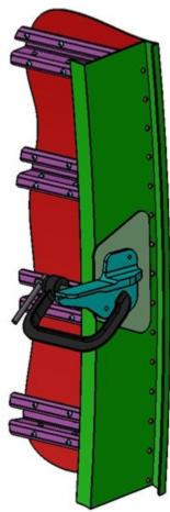
Figure 10 – Traditional: A part with pilot holes is clamped into position, not single-sided fastening
