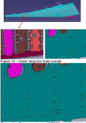
Figure 13 – Outer wing box build SSSF and drilled hole close-up.
