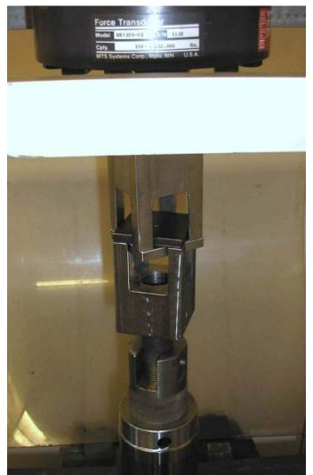
Figure 43. Star coupon testing in tension/compression machine.
