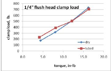
Figure 44. Clamp load versus torque for a Ø1/4, 100° countersunk SSSF.
