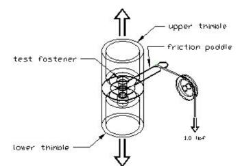
Figure 42. Tension testing per MIL-STD-1312-16
