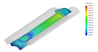
Figure 31. Maximum stresses during clamping – top view.
