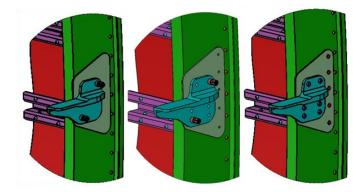
Figure 9 – Sequence of determinant clamp with SSSF, drill, and final fastening
