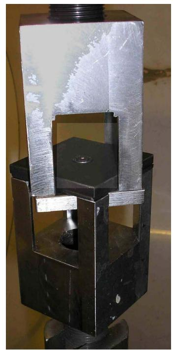
Figure 45. Fatigue test of a SSSF, head isometric view
