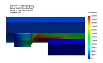
Figure 32. Maximum stresses during clamping.
