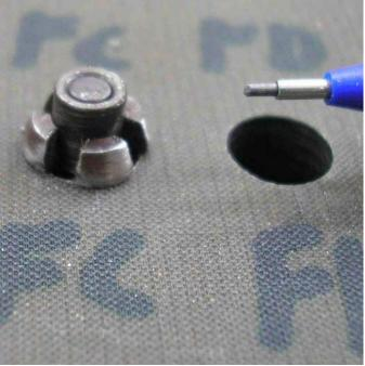
Figure 48. Tail-side hole specimen, during SSSF installation at 20 in-lb of torque
