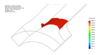
Figure 33. Volume of material that has exceeded yield levels during maximum clamping.
