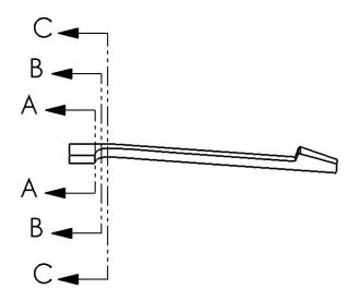
Figure 20. A single finger shown in the post heat treat condition depicted with multiple section planes.
