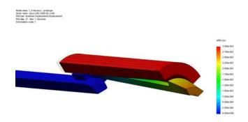
Figure 35. Residual deformation after Case 2A loading
