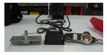
Figure 36. Test setup. Load cell with digital readout, SSSF ( $\emptyset$  1/4 inch), torque wrench. This is shown at the start of testing – fingers are only opened to trap the stack of 2 plates and the load cell.
