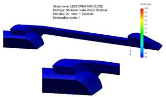
Figure 24. Case 1 loading does not cause residual stress or deflection after fingers close
