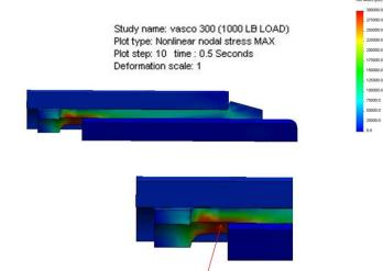
Figure 26. Maximum stresses during clamping.
