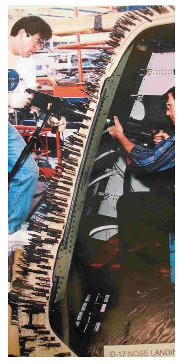
Figure 11 – Traditional: Many low-clamp force Clecos are needed for sufficient clamping (C17 nose landing gear door frame).
