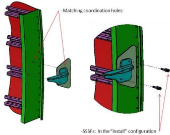
Figure 7 – Initial location during determinant assembly
