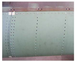
Figure 5. [1] High-curvature leading edge showing tack fasteners and drilled hole patterns
