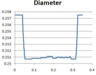
Figure 8. [2] Hole profile results using automated probe
