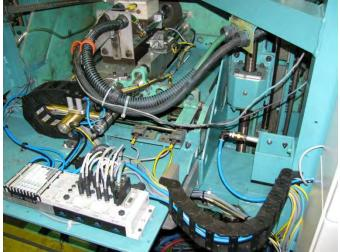
Figure 4 The Buca probe is the tool on the right of the wet side shuttle table.
