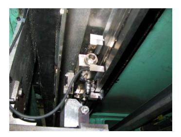
Figure 2: Installation of LM10 linear scale
