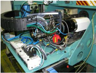
Figure 5 Precise drill spindle mounted on the new dry side shuttle table
