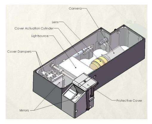
Figure 1: Bolt Camera Assembly
