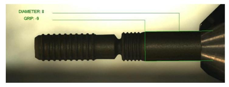
Figure 2: Operator Display of Measured Bolt Dimensions
