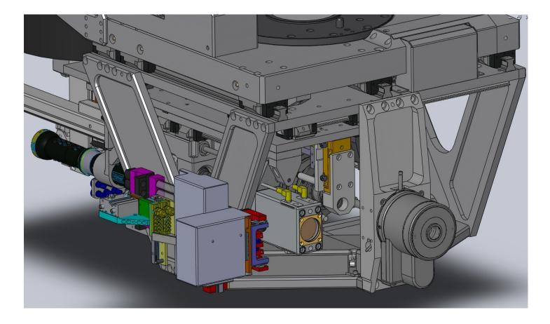
Figure 1: Aircraft Fastening/Drilling Machine End Effector
