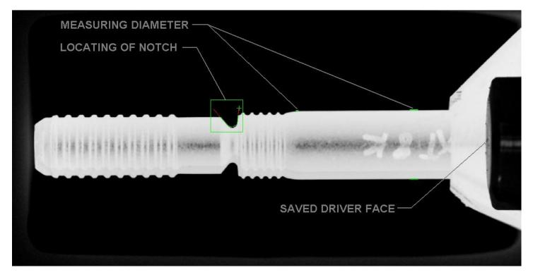
Figure 3: Measurement of Bolt
