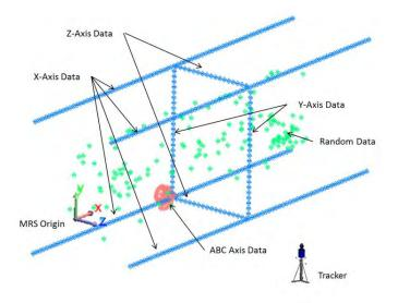
Figure 10 – X, Y, Z, A, B, C and Random Compensation Data
