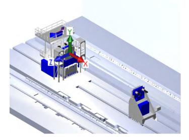
Figure 8 – Common Machine Coordinate System
