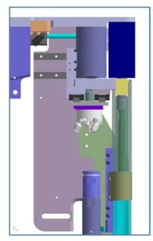
Figure 3. Bolt Impacts Polyurethane Rod
