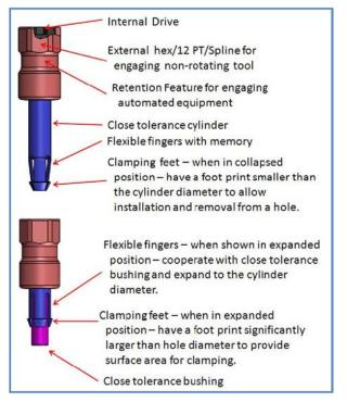
Figure 1. SSSF/SSTF Bolt Features. Adapted from [1]
