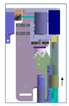
Figure 2. Bolt Entering Chamber
