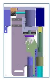
Figure 4. Damping Mechanism Retracted
