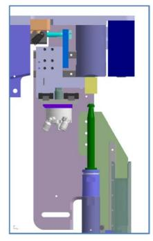
Figure 9. Bolt Inserter retracted with Bolt
