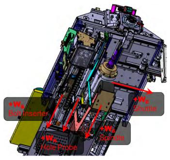
Figure 13. LTD process head with labeled process tool axes.
