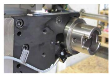
Figure 4. Single finger tool gripper shown with HSK 63A tool holder and proximity sensor.
