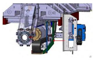
Figure 5. First gripper extends to receive tool from spindle.
