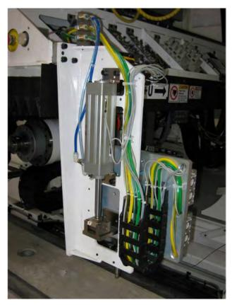
Figure 2. A two position air cylinder actuates to select gripper position.
