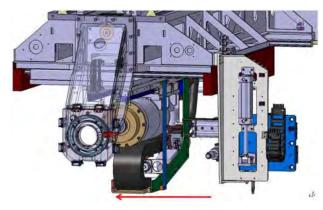
Figure 11. Shuttle movement unloads cutter from Position 1 gripper.
