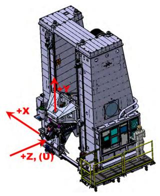
Figure 12. LTD shown with labeled major machine axes.
