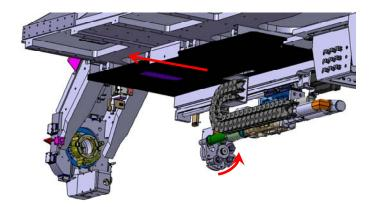
Figure 10-Bolt Inserter Advances Revolver
