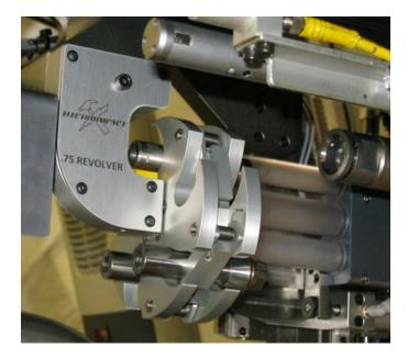
Figure 8-Revolver Feed Cartridge
