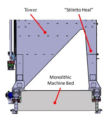
Figure 6-Tower on Monolithic Machine Bed
