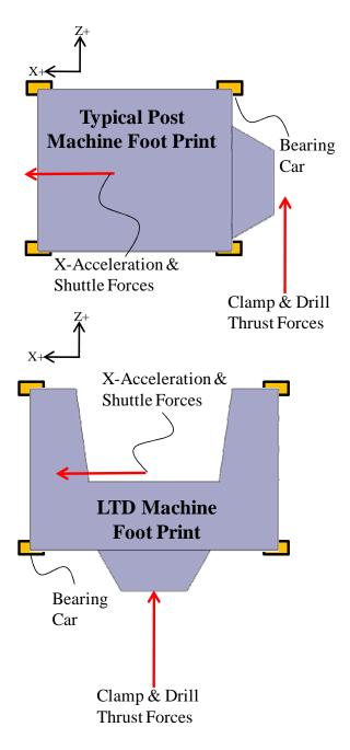
Figure 5-Comparison of Acceleration and Thrust Force Vectors
