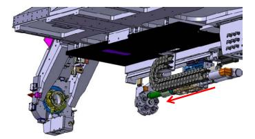
Figure 9-Bolt Inserter Engages Fastener
