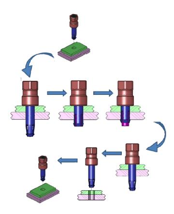
Figure 2-SSTF Clamping and Unclamping
